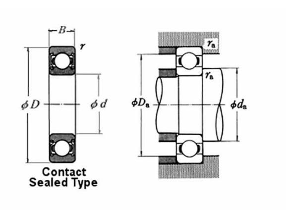
High quality Deep groove ball bearing with rubber contact seals from the world leader NSK, the worlds largest ball bearing manufacturer offering unparalelled quality. The unique & patented NSK DDU rubber seal features market leading technology, keeping contaminants and moisture out of the bearing while retaining the high class lubricant inside
